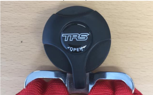
ALTERNATIVE ADJUSTER - PELVIC STRAP (ADJUSTABLE TONGUE - 24E0130)
