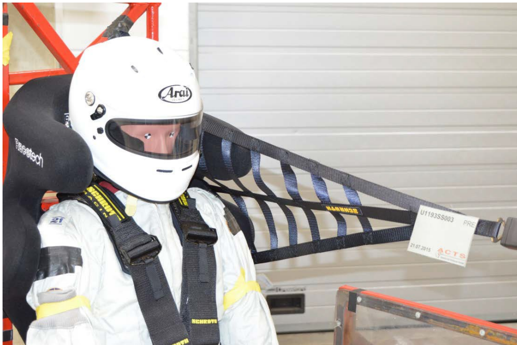
Figure 4 Z: Photograph showing upper-strap inside the seat-side-head, shown with single-front-attachment design (internal view, but valid also for dual-front attachment and door nets )
