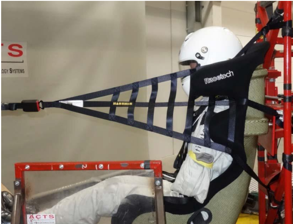
Figure 3: Photograph showing upper-strap inside the seat-side-head, shown with single-front-attachment design (external view, but valid also for Dual-front-attachment)
