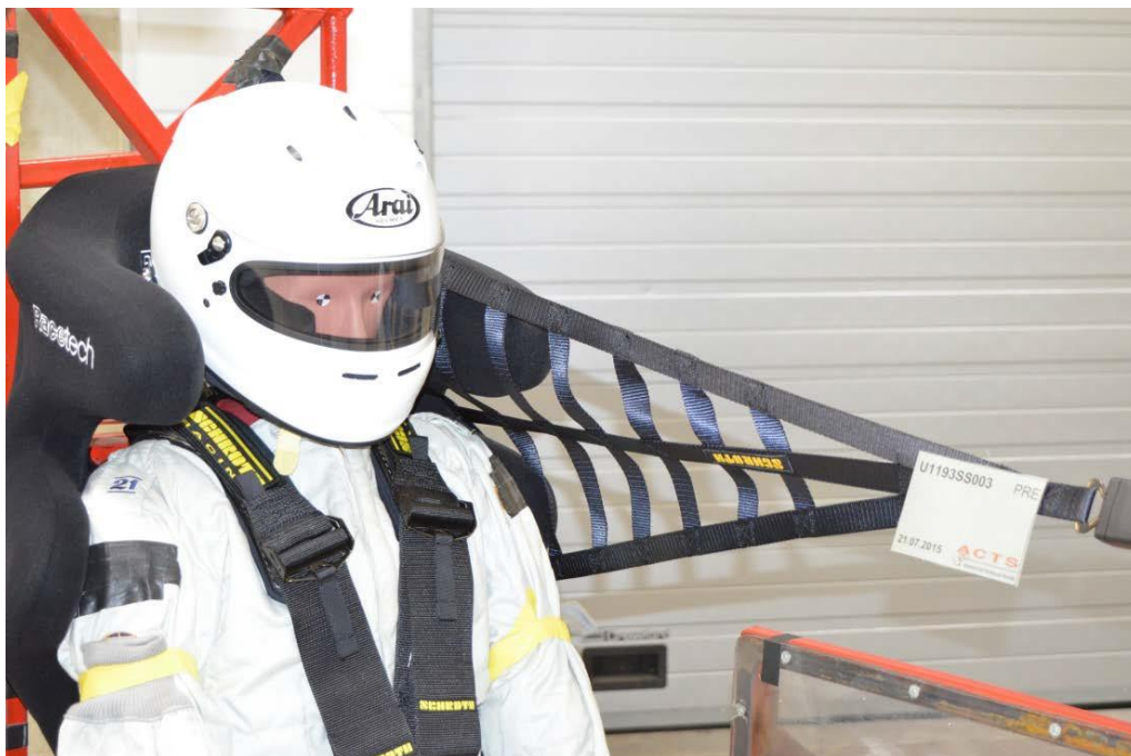
Figure 4: Photograph showing upper-strap inside the seat-side-head, shown with single-front-attachment design (internal view, but valid also for Dual-front-attachment)
