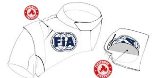
Figure 6 – Badge fixation (thread and backing flameproof)
