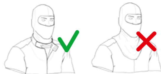
Figure 3 – Overlap of the overalls and balaclava
