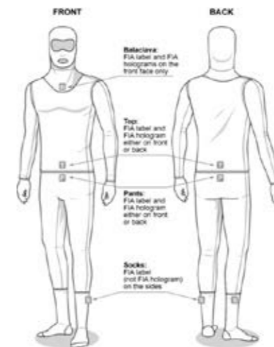
Figure 9 – Position of the FIA label on undergarment, socks and balaclava
