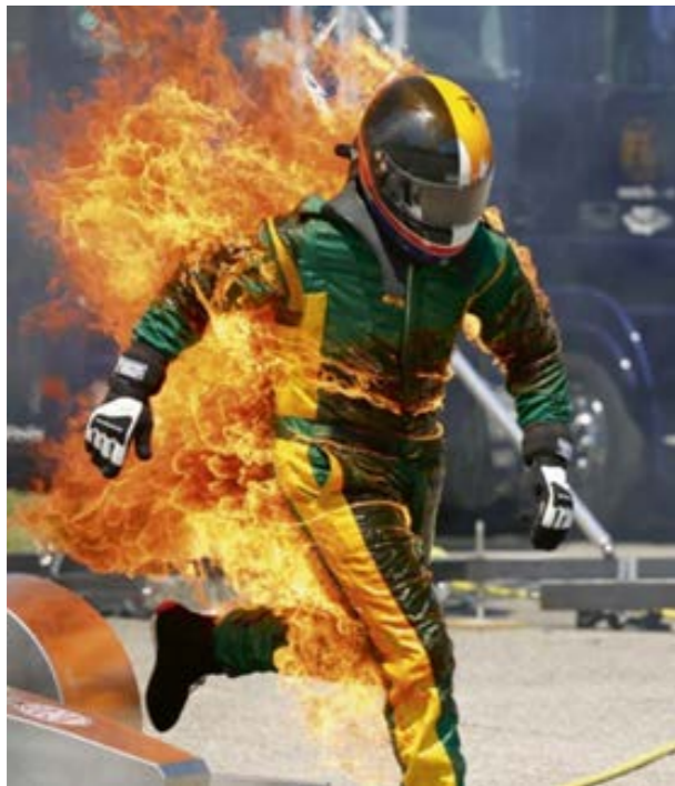
Figure 1 - Stunt man on fire equipped with FIA-approved clothing, helmet and FHR
