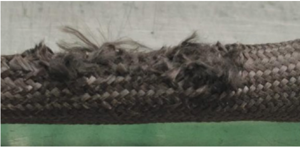
Figure 9 Damaged jacket of the restraint cable
