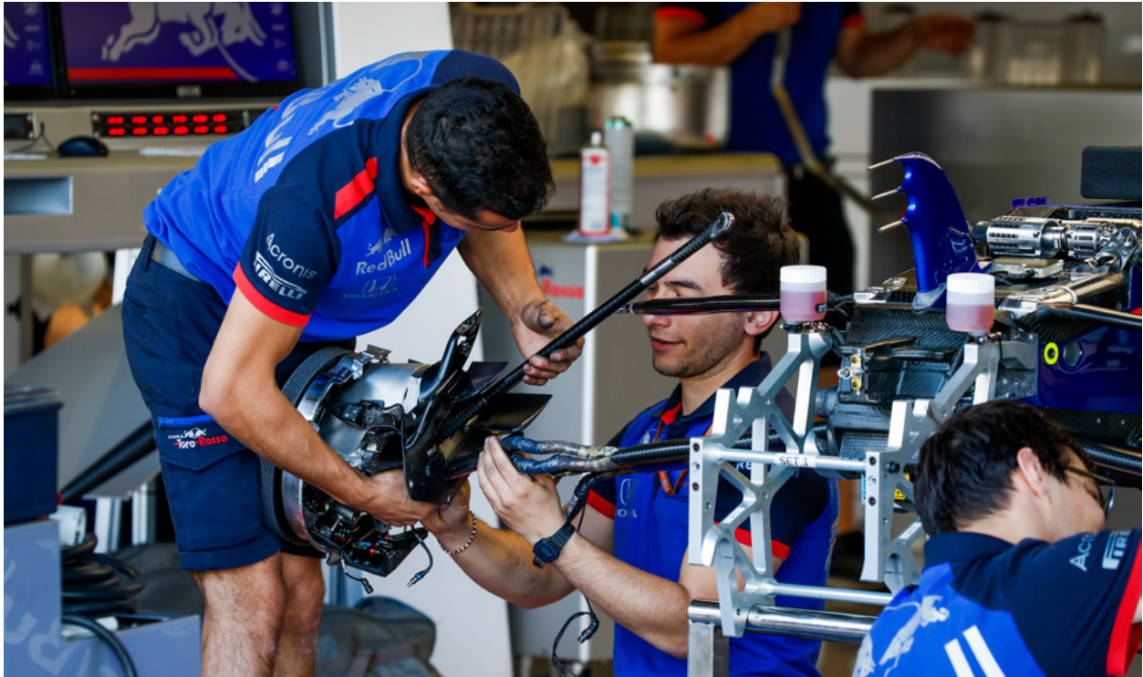
Figure 2 Installation in wishbones
