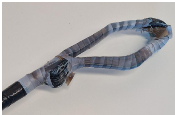
Figure 4 Restraint cable end fittings damage
