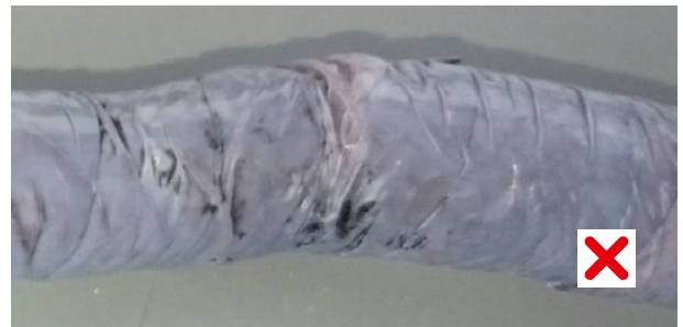
Figure 6 Liquid in contact with protective layer
