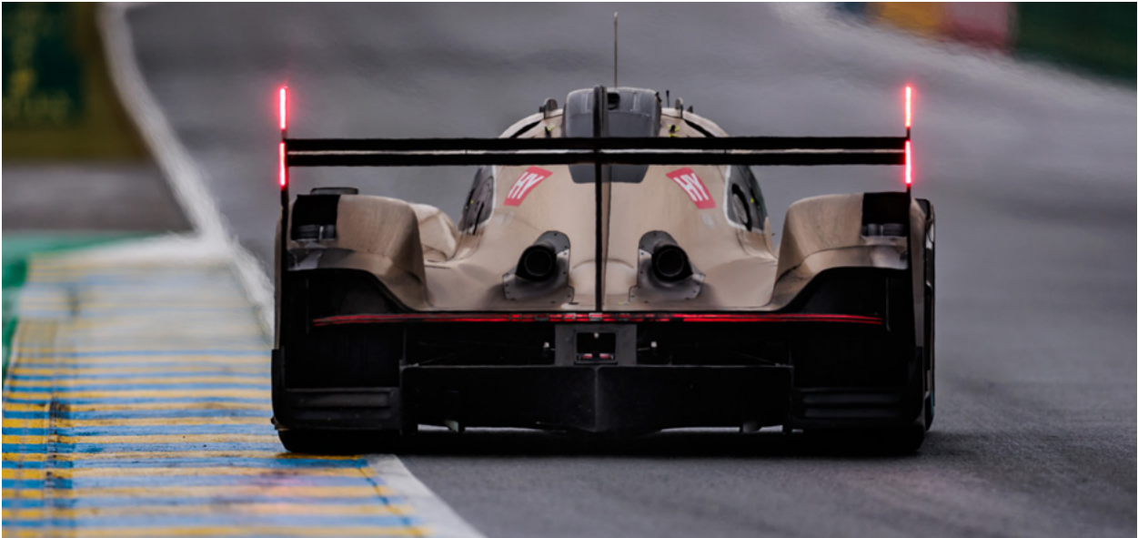
Figure 5 Vertical rain light configuration
