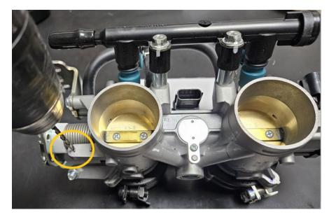
b) The original potentiometer fixing bolt must be replaced with a prepared M5x12mm Allen head bolt. A 2.5 mm hole must be drilled to the Allen head of the bolt.
