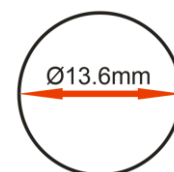
Figure 21 Activation Switch panel cut out
