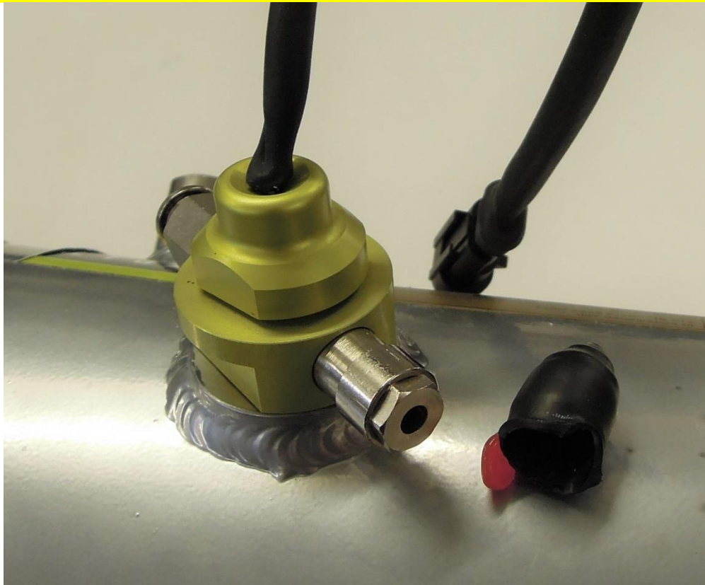
205. PHOTO DE L'INDICATEUR QUI MONTRE QUE LE SYSTEME DE DECHARGE DE PRESSION A ETE ACTIVE / PHOTO OF THE INDICATOR THAT SHOWS THAT THE PRESSURE RELEASE SYSTEM HAS BEEN ACTIVATED
