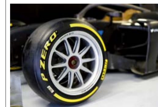
The new rules allow for new, wider 18-inch wheels, which will debut in the Formula 2 series in 2020.
