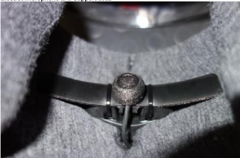
Electret Microphone and Support 2022
