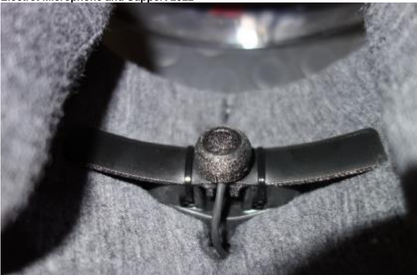
Electret Microphone and Support 2022
