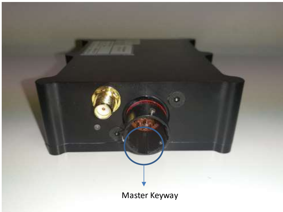
Figure 7 – Master keyway orientation
