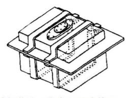
Cells without mounting flanges use 3x25mm straps top and bottom bolted or welded to frame in trunk.
