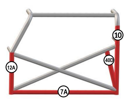
Panels must <u>not</u> be attached to rocker bar (7A), Windshield/Roof bar (12A), Main Hoop (10) or Driver side Kidney Bar (40D) if applicable.
