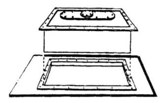
Weld 25mm tube frame to Trunk floor to bolt to cell frame.
