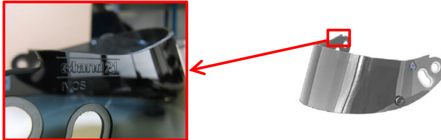
Figure 3 – Manufacturer and model engraved on visor
