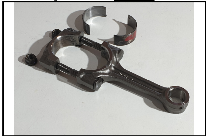
C5-2) Bielle de \frac{3}{4} arrière côté pied Connecting rod from \frac{3}{4} rear on small end side
