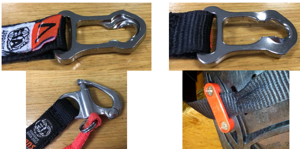
Figure 1 – Deformed end fitting (top right and left, and bottom left), and stretched FHR tether (bottom right)
