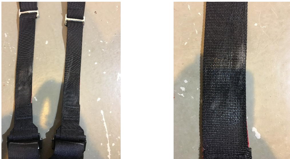
Figure 3 – Shoulder belts stretched after a severe crash
