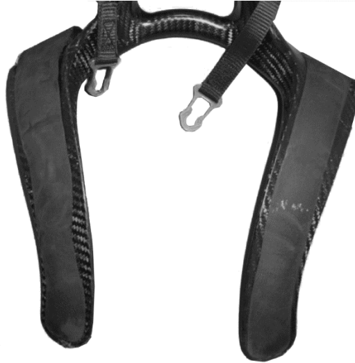
Figure 2 – Signs of wear on the rubber surface
