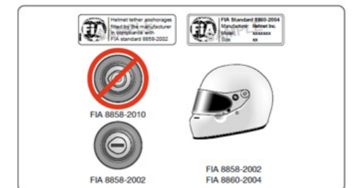
Fig. 27 - 8858-2002 Helmet-M6-anchorage – can only be used with FIA-approved 8858-2002 helmets (Technical List No. 41 – Part 2)
