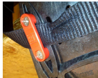
Fig. 29 – Deformed end fitting (top right and left, and bottom left), and stretched FHR tether (bottom right)
