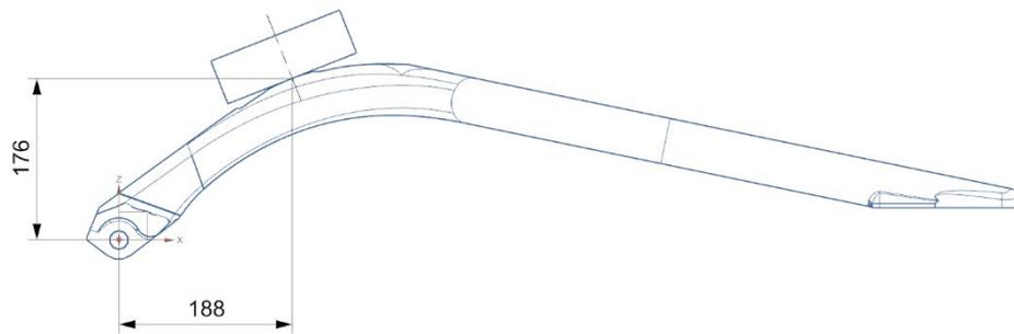
Figure A3.4.1 Load application point for Static Test 1
