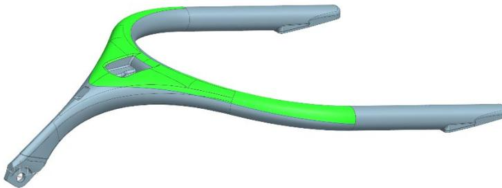
*Wall thickness  $\geq$  3mm in green area*
